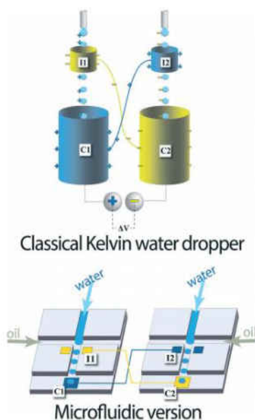
Fig. 25. Schematic of the microfluidic Kelvin water dropper[42].
